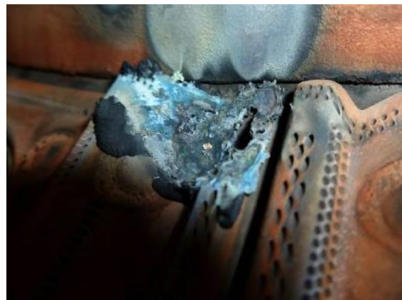
Figure 24 - ABK RB 211 Front Combustion Liner not Re-Usable after 6,800 Running Hours and Low Grade F7 Filtration –
