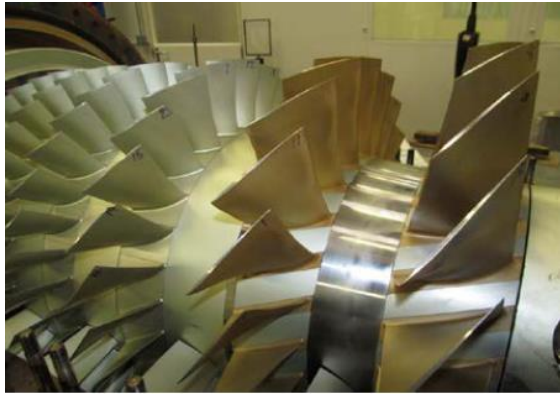
Figure 19 - ABK SGT400 Compressor Cleanliness after 5300 Running Hours with the Retrofitted E12 Filtration Grade -
